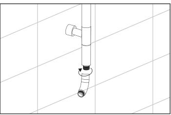
Screw swivel joint (7) onto shower bar.
