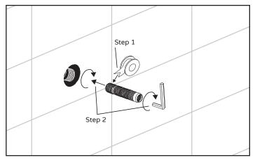
Screw nipple extension (5) into pipe. Make sure you have 1/2" off the wall.
