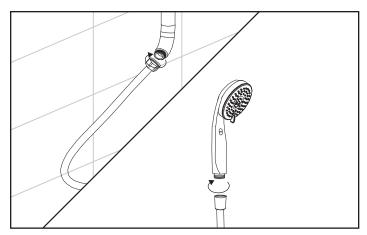
Attach hex head end of hose (12) to swivel joint (7) and tapered end to hand held shower (11).
