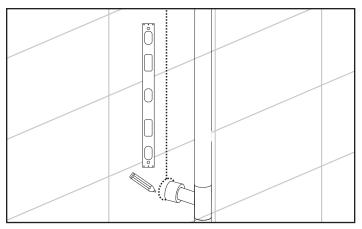
Use level to assure shower pipe is straight. Mark desired location for bottom mount (9).
